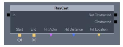
Performs a ray-cast from the starting point to the end point, determines if anything was hit along the way, and fires the associated output socket. The first hit actor is returned as well as the distance to the hit object and the location of the hit. The ray-cast ignores the actor that contains the starting point.
