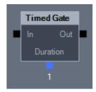
This action allows you to pass through a signal to the Out signal out socket depending on the state of the gate. The gate is automatically closed for the specified time when a signal pass through the gate.
